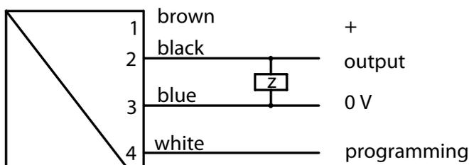
The correct supply voltage value acc. to datasheet values has to be obeyed prior to installation! The use of shielded cable is highly recommended, cable length < 30 m, supply lines < 10m.
